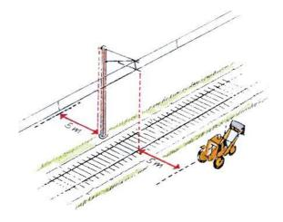
Large machinery must be protected to ensure that no part of it can get closer than 5 metres to voltage-carrying structures - even by accident or by making a wrong move.
