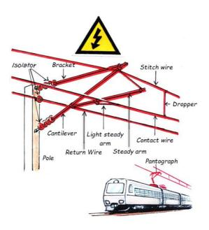
Please note that the return wire (on the S-train line conductor) has the same voltage as the overhead catenary.
