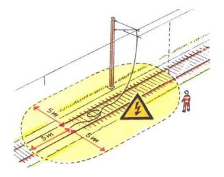
The safe distance applies until the catenary system technicians have ensured that the lines are without voltage and earthed for work purposes.
