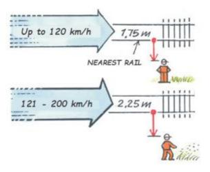
When moving and staying on platforms, there are special safety distances that must be observed.
