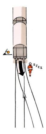
Never move between the buffers if you need to pass a stationary set of carriages. Use the safe way detour - go all the way around the carriages.
